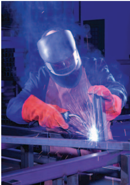
MIG/MAG-torch without fume extraction
